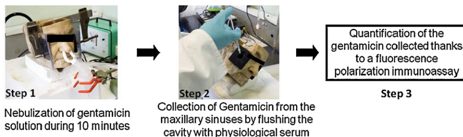
Fig. 2. Overall description of the drug deposition assessment procedure on the plastinated nasal cast.
